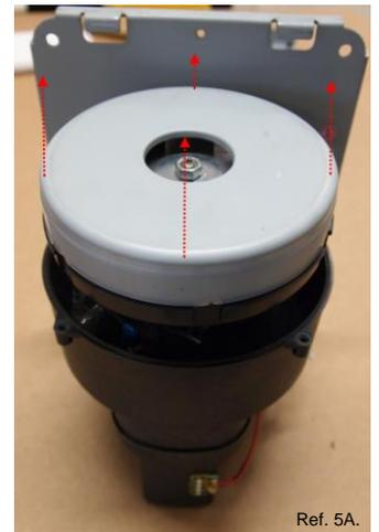
Disconnect motor wires from the timer unit (cf. photo ref. 5C or photo ref. 5D depending on timer unit type). Place the motor on a table - upside-down.
