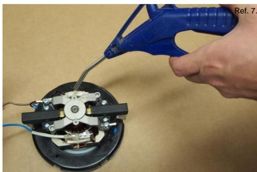
8. Blow clean motor housing – both top and bottom parts.
