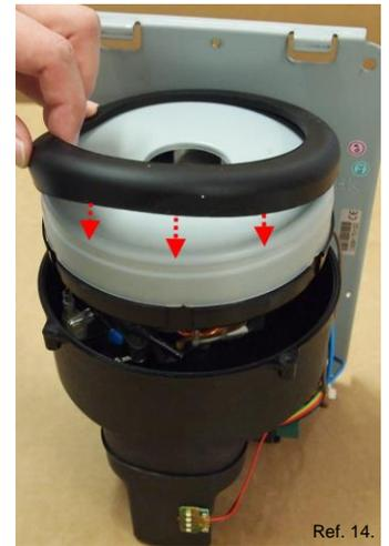
Assemble the top of the fan housing onto the bottom part by tightening the four screws – being careful not to overtighten. Fix angle bracket to base plate (cf. photo ref. 15B).
